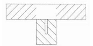
**10** Complete the sketch to show the construction of blockboard.
